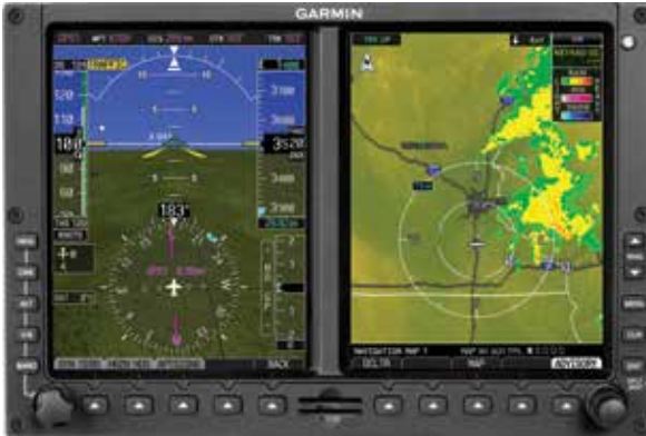
Figure 1-2 GDU 620 PFD and MFD
