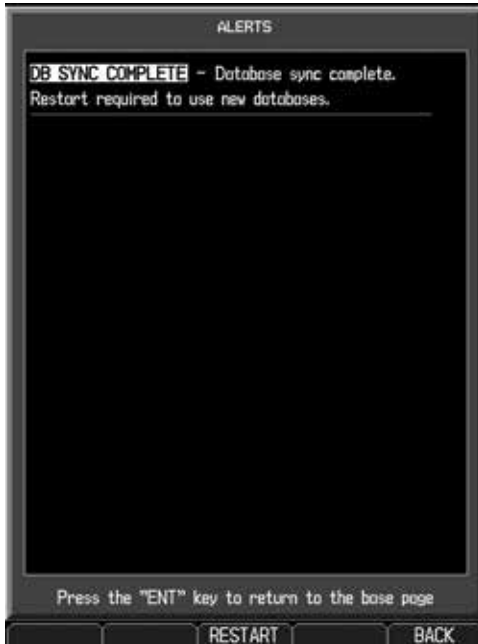
Figure 3-59 System Restart - Step 1
