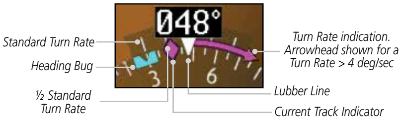
Figure 2-29 Turn Rate Indicator and Trend Vector
