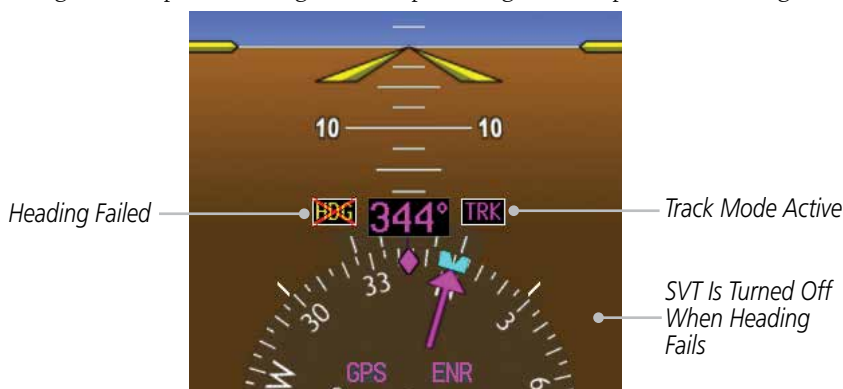
Figure 1-7 Track Mode shown as Active when Heading Info has failed
